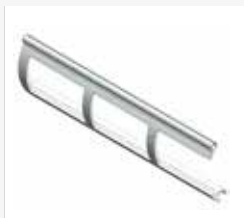
Slat 50 large hole 2560 , profiles 50 mm extruded aluminum, die cut hole 60x34 mm, suitable for outdoor use.
